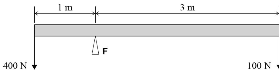
What is the reaction force acting on the rod at support **F**?
